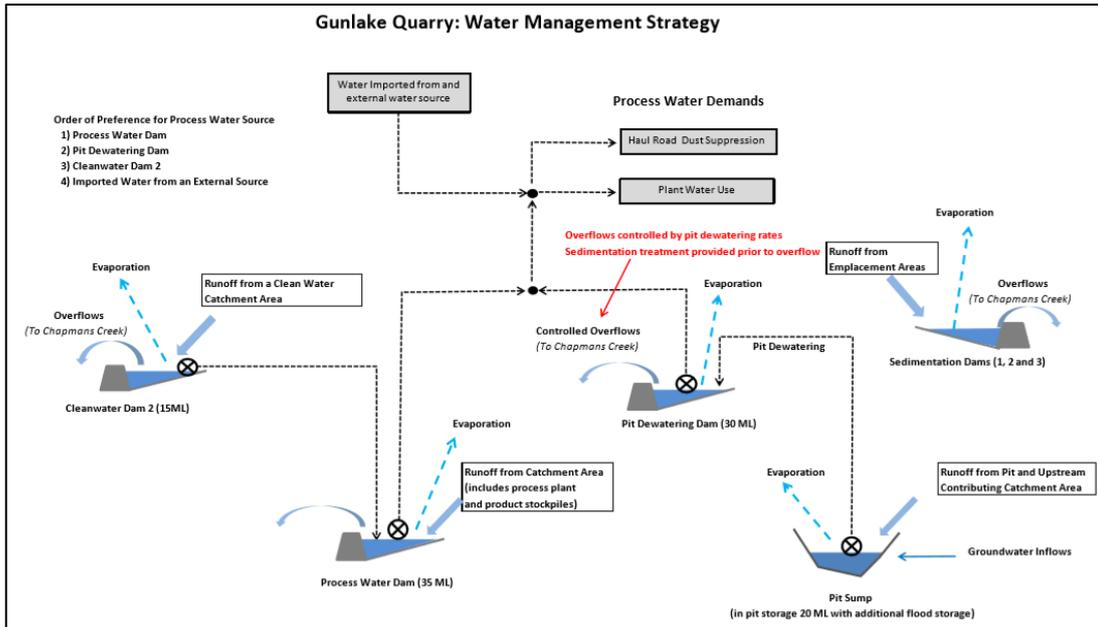
**Plate 7 – Surface Water Management Plan**
